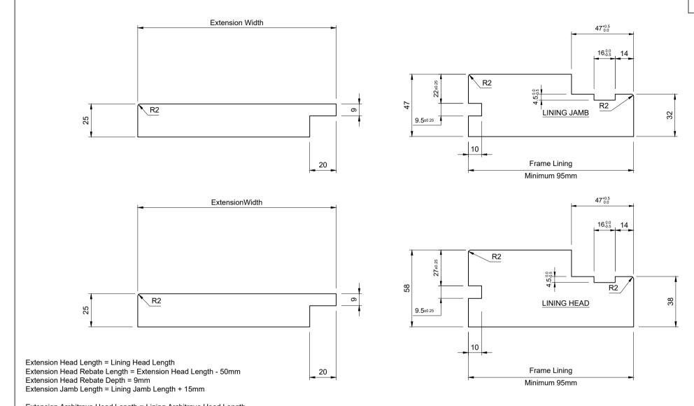
Extension Architrave Head Length = Lining Architrave Head Length Extension Architrave Jamb Length = Lining Architrave Jamb Length
